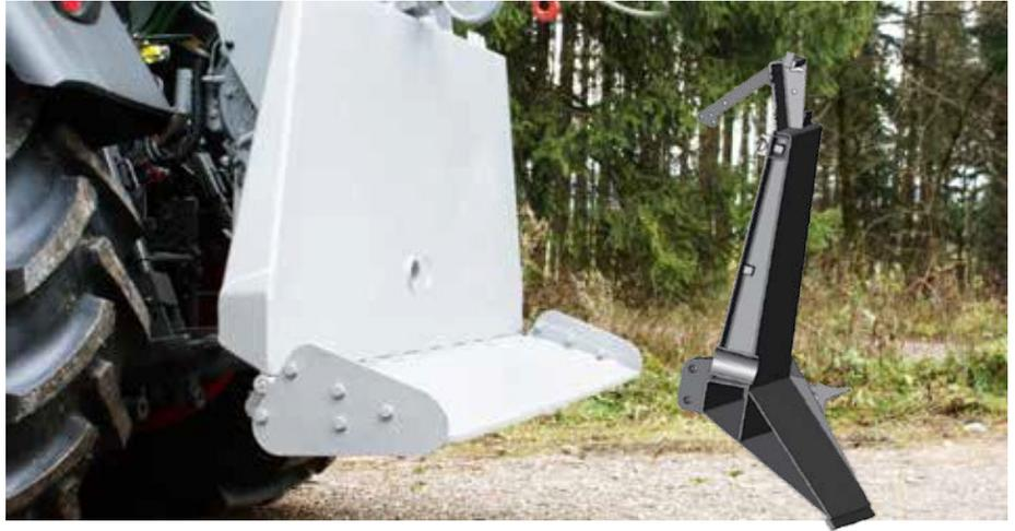
In addition to 3-point attachment, the cable winch can also be mounted via a **4-point attachment**. This guarantees the highest degree of stability. The Pfanzelt attachment system facilitates rapid and simple attachment.
